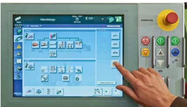
Fig. 7. Touchscreen control panel on a weaving machine [19]
