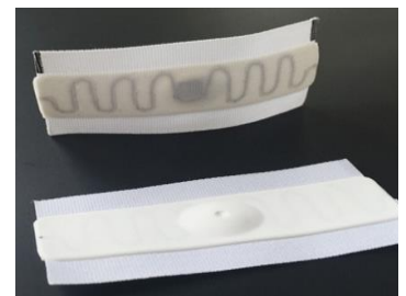
Fig. 8. Washable RFID tag used in textile cleaning
